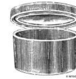
No. 677 - Stender Dish or Preparation Jar 1903 Number: No. 0 - Preparation Jar or Stender Dish.
